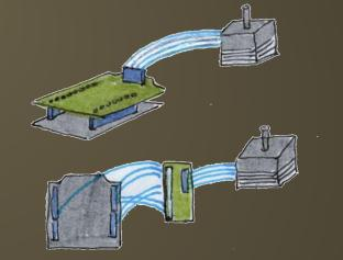
• Use standard pin-outs and keyed/unidirectional connectors to minimize inverted connections
